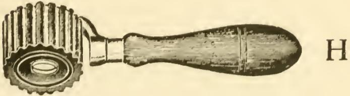
Fig. 51. Paperhanger's Seam Rollers.
