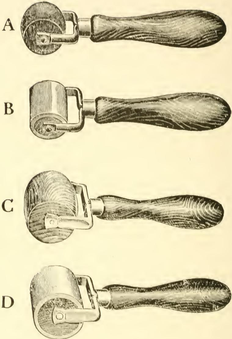
Fig. 50. Paperhanger's Seam Rollers.
